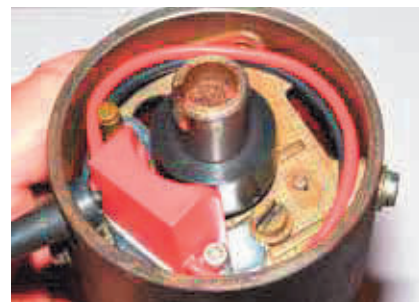
Giveren (magnetring) monteret
